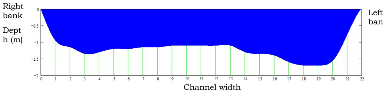
Figure 8: Active section on Timiș River to Grăniceri.
